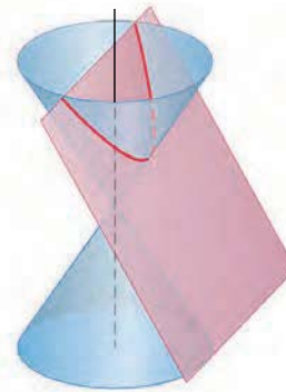
Parabola: plane parallel to side of cone
