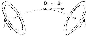
FIG. 10-14. Axial nature of the field in a toroidal winding is shown by combining the magnetic field of the current loops in pairs.
